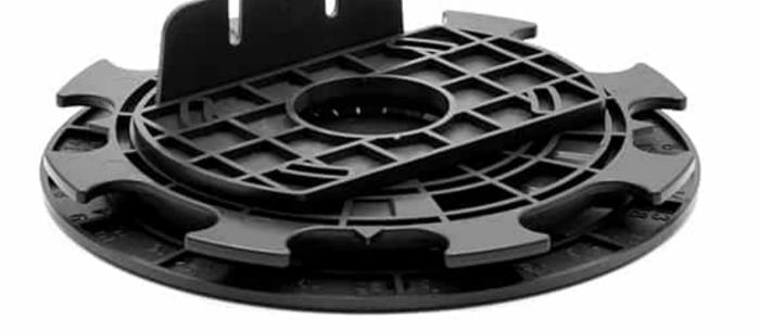
The adjustable decking pedestal from 8 to 20 mm allows the installation of a low height terrace. It can be adjusted from 8 to 15 mm without the wedge or up to 20 mm with. It is ideal for creating a roof top or covering an existing terrace.
